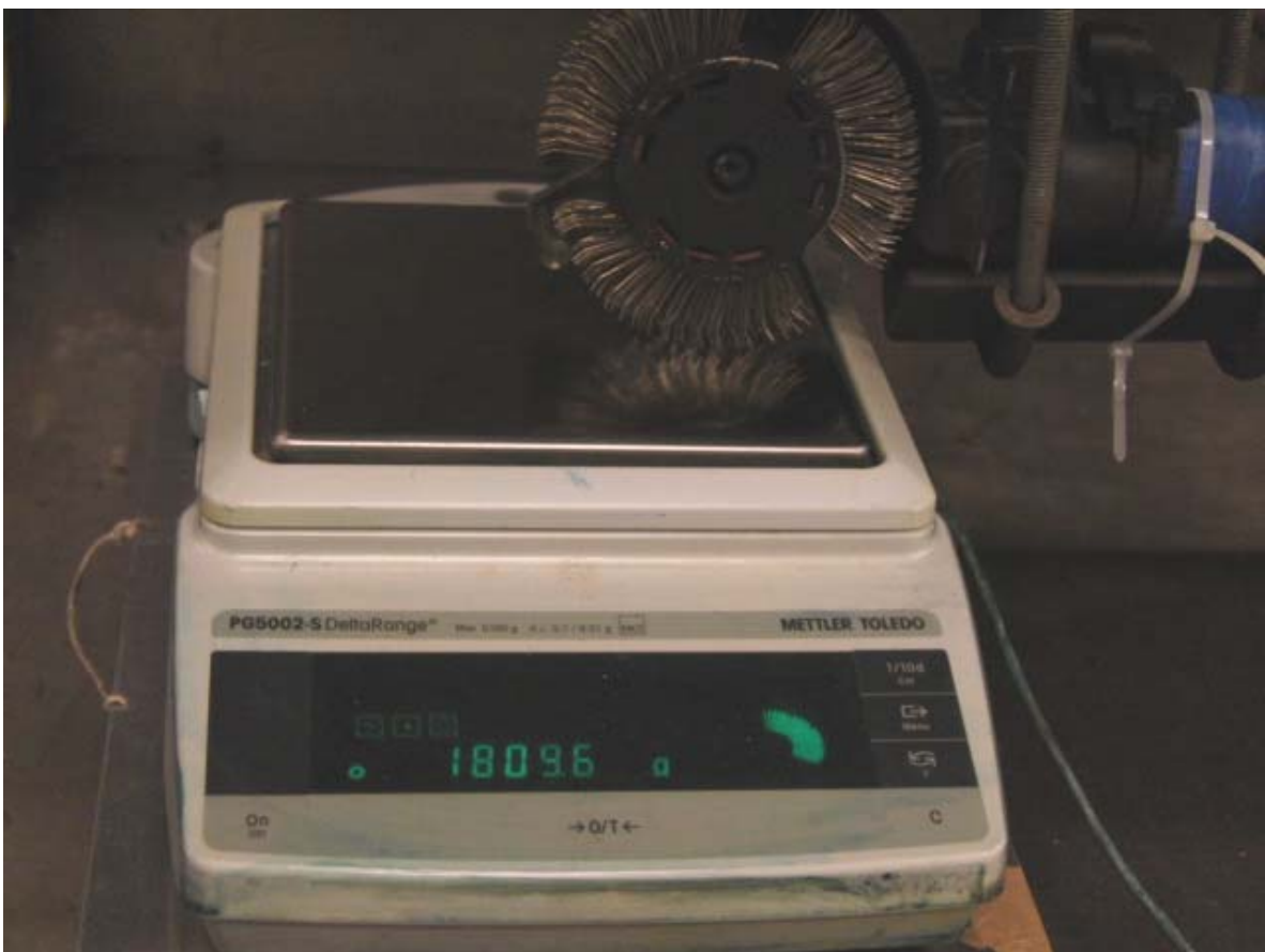
Figure 2.5 Measurement of the load applied to the tool when using the robot arm.
