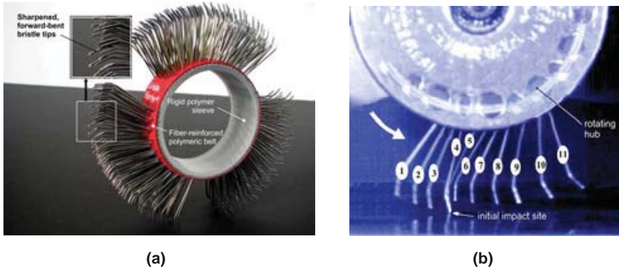
Figure 6 (a) Design and construction of the bristle blasting tool, and (b) successive frames of a single bristle taken from high-speed digital camera depicting the approach (frames 1, 2, and 3), contact/collision (frame 4), subsequent retraction (frame 5), and return to equilibrium position (frames 6-11) of bristle
